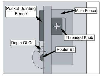
Figure 19. Proper setup for jointing an edge.
